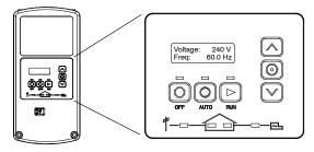
The RDC2 controller provides integrated control for the generator set, Kohler<sup>®</sup> Model RXT transfer switch, programmable interface module (PIM), and load management.
